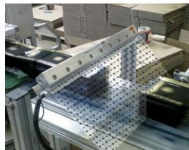
The Model 111118 18" (457mm) Super Ion Air Knife System eliminates dust from body care products prior to sealing the boxes in cellophane.
